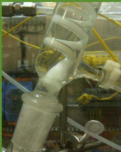
Scaling in the overhead during regeneration
